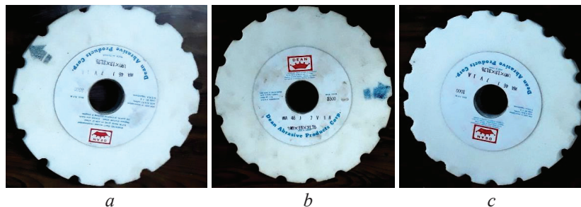
Fig. 1. Experimental segmented grinding wheels: a – 15 grooves, b – 18 grooves, c – 20 grooves
