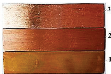
Fig. 3. Research results of corrosiveness fuel tests: 1 – E-85 (basic formulation), 2 – E-85+CNOs, 3 – isooctane (standard)
