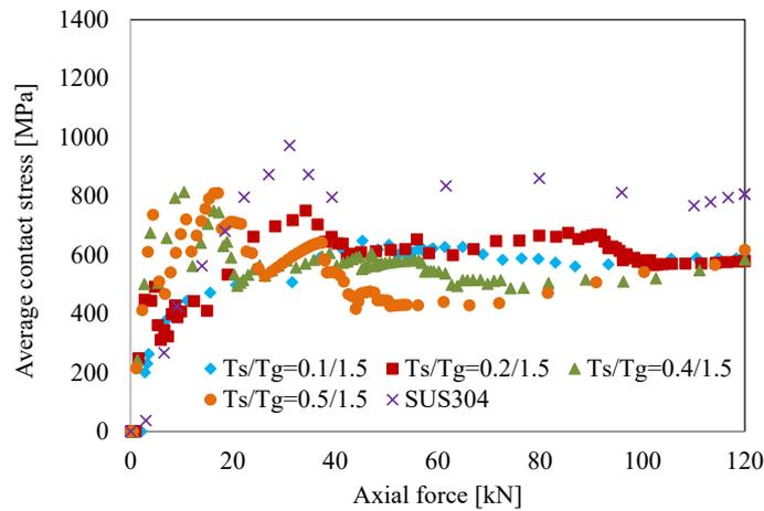
Fig. 15. Gasket contact stress in 400-MPa mode [3.5 μm]
