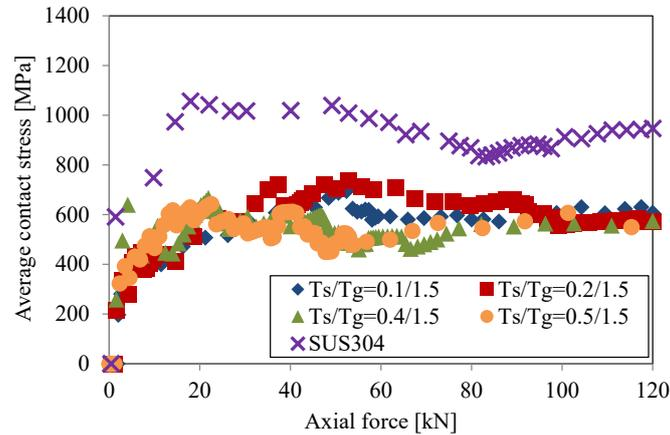
Fig. 17. Gasket average contact stress [2.5  $\mu\text{m}$ ]
