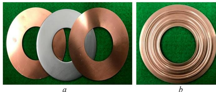
Fig. 8. Three-layer metal gasket: *a* – before forming; *b* – after forming
