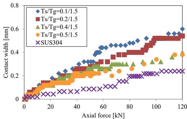
Fig. 16. Gasket contact width [2.5 μm]
