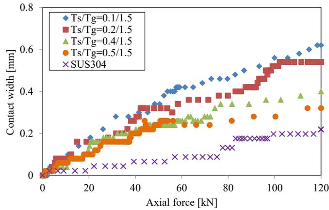
Fig. 14. Contact width for a gasket in 400-MPa mode [3.5 μm]
