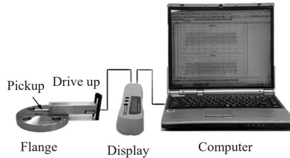
**Fig. 9.** Measurement setup for surface roughness
