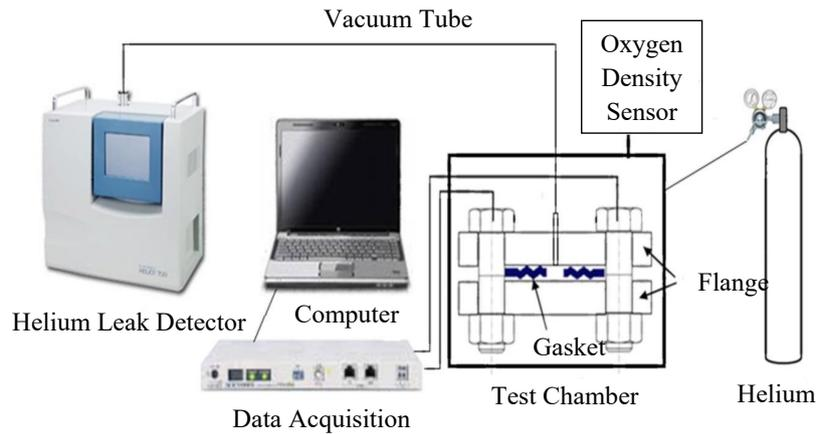
Fig. 12. A helium leak detection system design
