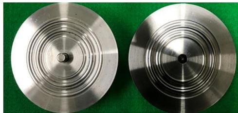
Fig. 7. The upper and lower dies
