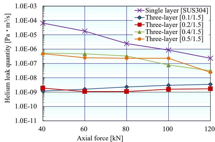
Fig. 18. Helium leak quantity test result (Ra 3.5  $\mu\text{m}$ )
