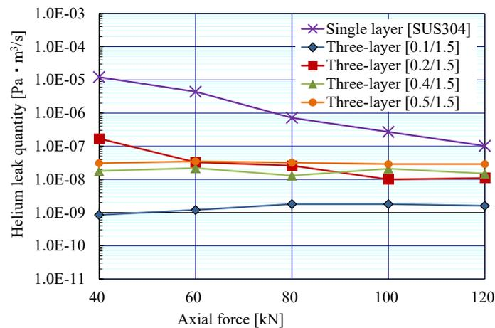
Fig. 19. Helium leak quantity (Ra 2.5  $\mu\text{m}$ )
