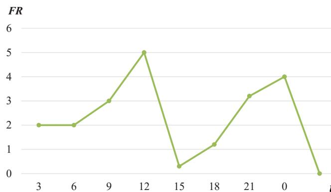
**Fig. 1.** Dependence of the frequency ranges of the signals of the ground-based ionosphere radiosounding complex on the time of its use:  $FR$  – frequency ranges;  $t$  – time
