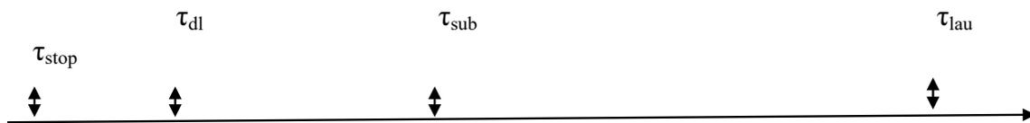
**Fig. 4.** Diagram of the preparation cycle for starting and stopping a measurement session in time:  $\tau_{lau}$  – the launch time of the complex;  $\tau_{dl}$  – the delay time of the start;  $\tau_{sub}$  – the launch of the substation;  $\tau_{stop}$  – stopping the operation of the entire complex
