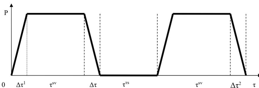
**Fig. 5.** Time diagram of the pneumatic actuator work:  $\Delta\tau^1$  – rod pushing out time;  $\tau^{sv}$  – idle time according to technological standards;  $\Delta\tau^2$  – rod pulling in time;  $\tau^{TS}$  – technological shutdown time
