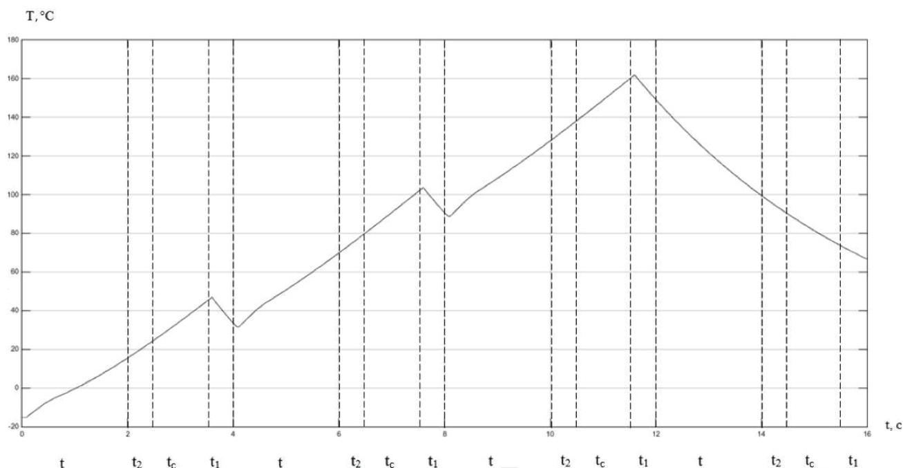
Fig. 7. Fragment of experimental research results:  $t$  – technical waiting time;  $t_2$  – time of extension of the rod of the pneumatic cylinder;  $t_1$  – return time of the pneumatic cylinder;  $t_c$  – cast time
