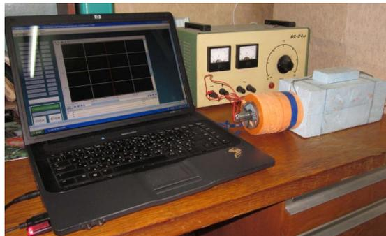
**Fig. 1.** Laboratory low-temperature calorimeter with analogous-digital transformers, produced by DCON Utility (USA)
