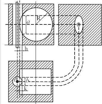
**Fig. 1.** Projections of two connected hollow cylindrical structures
