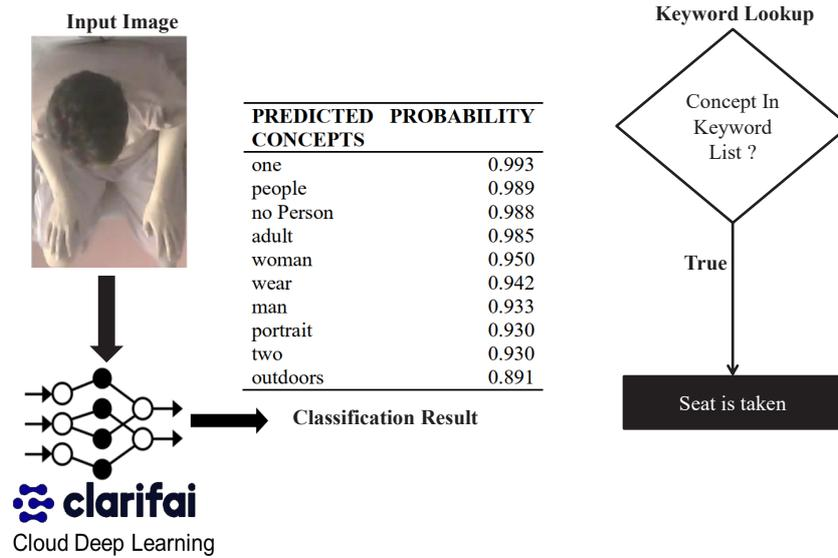
Fig. 3. Seat availability detection mechanism
