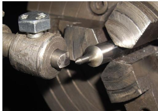
**Fig. 6.** Pre-installation of the mandrel for diamond knurling
