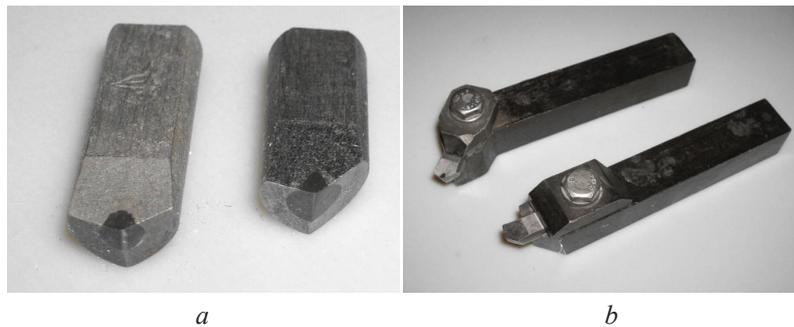
**Fig. 1.** Turning cutters with cutting material made of superhard materials:
