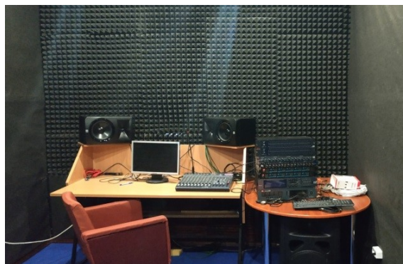
Fig. 1. Silenced room of the Department of Acoustic and Multimedia Electronic Systems NTUU “Igor Sikorsky Kyiv Polytechnic Institute” to study the effect of complex audio signals on the electrical activity of the human cerebral cortex
