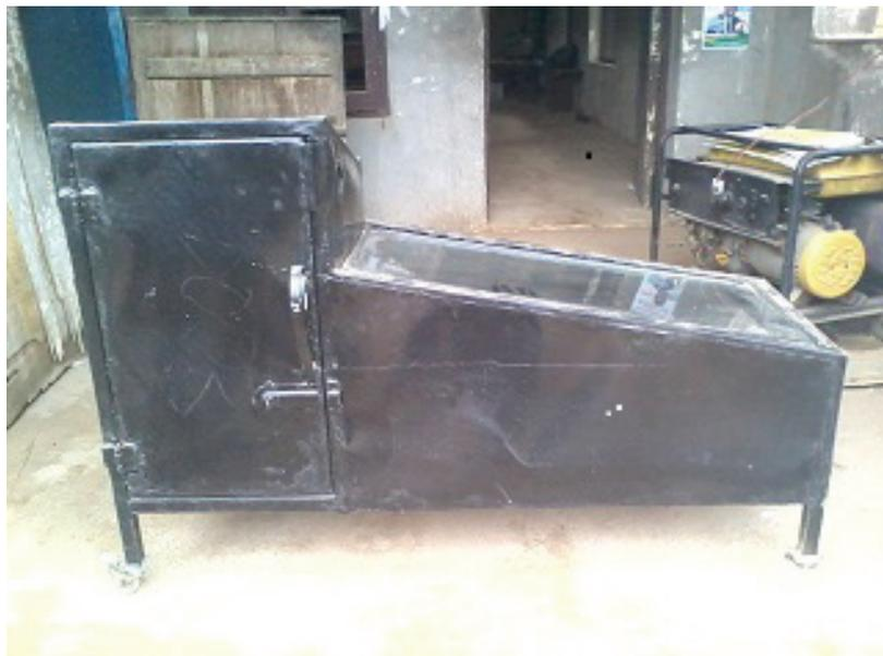
**Fig. 2.** The designed solar dryer
